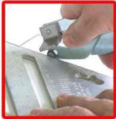
For Straight Lines, either draw a line with a marker and follow it by looking at the back of the scoring wheel and following it as you score, or run the flat side of the wheel against a speed square or thick straight edge held or clamped down firmly, don't use another tile or piece of wood, they are not smooth and will grab and prevent the wheel getting a good score. If you are left-handed remember to flip the wheel to the other side so you can see it.
