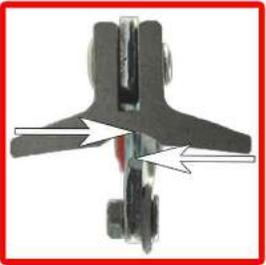
If the breaker is too loose you can tighten the rivet by placing the head of the rivet on a solid surface and hitting the open side of the rivet with a ball peined hammer to squeeze the aluminum to the metal handles. If you are only using it for thin glass all the time you can superglue the aluminum breaker so it stays in that position permanently.
