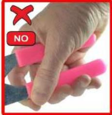
Holding the Tool Incorrectly, i.e. by the Handles while scoring Will Not apply anywhere near enough pressure onto the Scoring Wheel and will prevent the tool from working efficiently. Holding the tool way back there like this will also require a lot more strength to score as you do not have any leverage, and you will not be able to make the tool do what it is supposed to do, the handles are just for squeezing once the material has been scored correctly, and not for holding while scoring.
