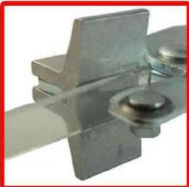
It will always be easier to cut a strip in half than trying to cut a strip off the edge of a piece of glass, for example if you want a quarter inch strip in 1/16" thick glass, instead of trying to cut a quarter inch strip off the edge of the edge, first cut a half inch strip off then cut that piece in half. The stress in the glass is equalled out when each side is similar in width, as it takes even pressure to bend both sides and bending it is what we are actually doing when we break it.
