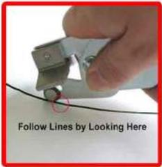
Radius / Curved cuts can be made by drawing a line and following the line by looking at the back of the wheel as you score very firmly. Up to a quarter of a circle can be cut in a single cut, to do a semi-circle we saw a straight line down the center, then we can score and break two quarter circles. For Wall Tiles you can saw using the Rodsaw in a Hacksaw and to saw through Floor Tiles and Porcelains use one our Diamond Grinder Blade in an Angle Grinder.
