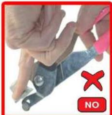
This shows an incorrect two handed method for scoring Floor Tiles, although two hands are being used, the strongest hand has been moved back and is now holding the handles and not applying any pressure at all to the wheel, so now we only have the weakest hand applying pressure to the wheel, whilst this might work for Wall Tile and Glass it will definitely not work for scoring Hard Tiles Like Floor Tiles & Porcelains.
