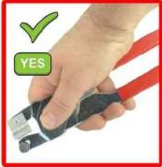
Holding the Tile & Glass Cutter the correct way is an absolute must, always hold it as close to the Scoring Wheel as possible when scoring, this not only gives more pressure, it gives a lot more control. If you get into the habit of picking it up by the center rivet between your finger and thumb, then wrap your hand around it you will always be holding it correctly. Yes It really does matter.
