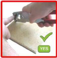
With Floor Tiles and Porcelains use the two-hand method, this gives you the extra pressure needed for those hard and thicker tiles. A bench or solid table at waist height with a wooden or MDF board on top makes a great cutting surface, this allows you to lean over to apply more pressure using your upper body weight. Running off the edge of the tiles at the end of the score and hitting a wooden board below will not do damage to the wheel and it will ensure you score all the way to the edge.
