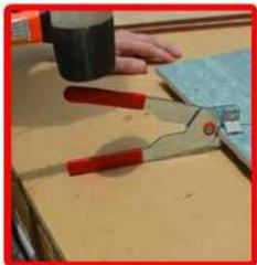
If you have scored the tile hard enough but cannot physically squeeze it, you can line the tool up as though you were going to squeeze it, sit it down on a solid surface, and give it a sharp tap with a mallet or hammer. Using the side of the hammer instead of the face will give a wider contact area and less chance of missing it etc. This is how we cut the thick Quarry Tiles in our live demonstrations. It also demonstrates how tough the tool is.
